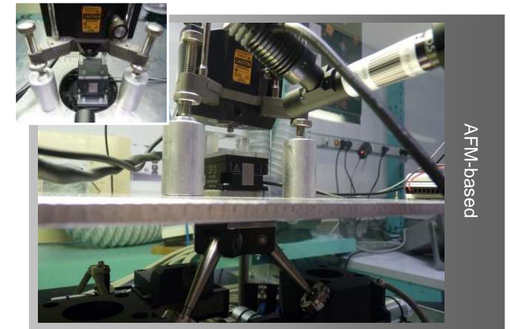
Micro-force measurement multimodal platform using an AFM cantilever
